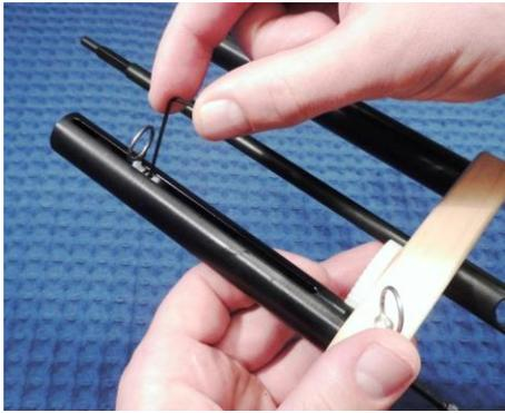
Using the Allen wrench, loosen the set screw which holds the moving eyelet in place. Loosen it 1 to 1 1/2 turns. Do not completely remove the set screw as it is very easy to lose.
