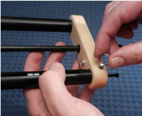
Screw the stationary eyelet into place. Tighten it only enough to properly position it. Over-tightening can make it difficult to remove and may damage your winder.
