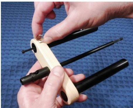
Using your fingers, unscrew and remove the stationary eyelet from the flier base. If it is too tight, try putting a pencil through the eyelet and then turn the eyelet with the pencil.
