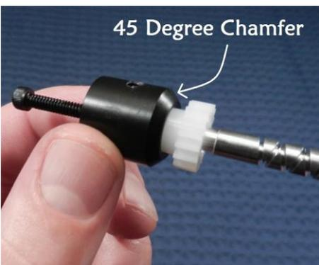
The black front bearing has one end that has a sharp edge and the other side has a 45-degree chamfer cut into it. Slip the front bearing over the hub of the small gear with the 45-degree chamfered end toward the gear teeth.
