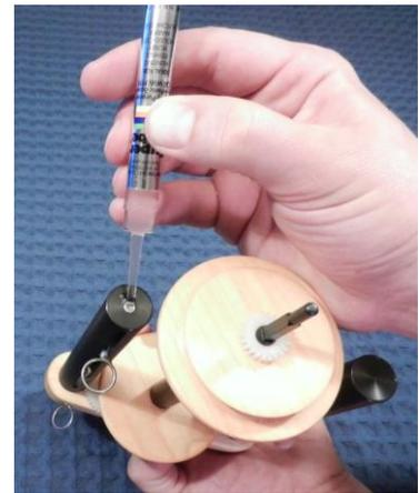
On each end of the flyer shaft where the bobbin gears ride on the shaft, a light application of any grease or Vaseline should ensure that the bobbin winds freely and without noise. You can use oil here as well; however, the grease is better at preventing any bobbin knocking noise.
