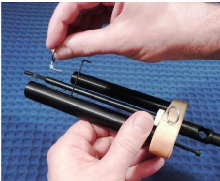
Remove the eyelet by sliding it away from the base of the flier. Make sure the little white "Quiet-Glide" bushing does not fall into the travel arm.
