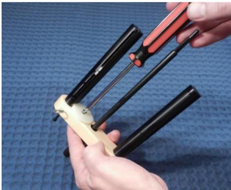
With a household screwdriver, remove the large gear.
