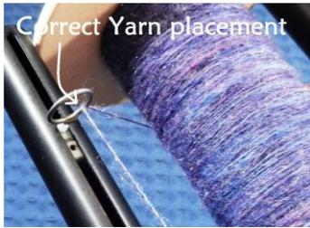
If your yarn should suddenly fail to wind onto the bobbin, first check the yarn to make sure it hasn't flipped itself around the moving eyelet. This occurs occasionally when all tension is released on the yarn i.e. if you treadle backwards when starting.
