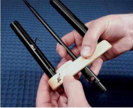
Turn the large gear until the set screw for the moving eyelet is visible. Insert the Allen wrench and loosen the screw 1 to 1½ turns. Leave the Allen wrench in place.
