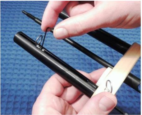
Use the Allen wrench again to tighten the set screw so that it will hold the eyelet in place. Don't over tighten it -- just snug will do fine.
