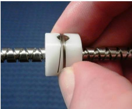
To remove the coil spring that is wrapped around the traveler, locate the end of the spring that is nearest to the small gear. With your fingernail gently lift and push the end of the spring until it is off the traveler. Guide the rest of the spring with your finger while turning the traveler so as to unscrew the spring from the traveler.
