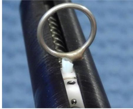
When the eyelet and bushing are properly installed, the bushing will be completely on top of the white traveler.
