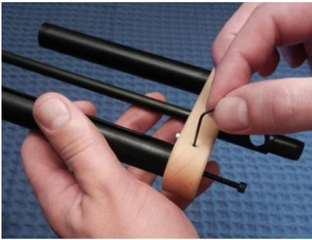
Use the Allen wrench from the tool kit to verify that the hole in the end bearing is lined up with the hole in the flyer base. Insert the Allen wrench into the eyelet hole and move the Allen wrench in a circle. The Allen wrench should go through both parts which will ensure that the two parts are properly aligned for the next step.
